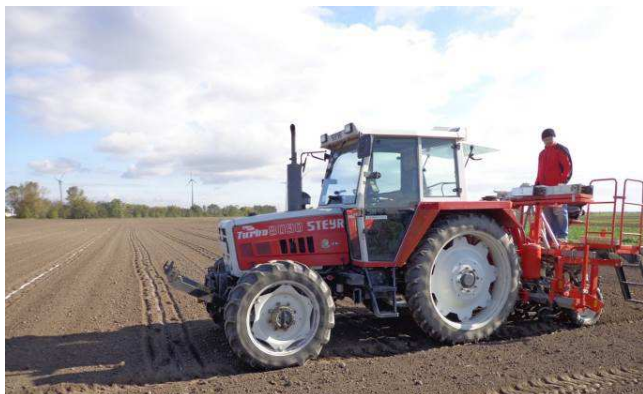
Sowing of spelt wheat in mid-October 2014 in Austria using a Hege pneumatic single seed sowing machine
